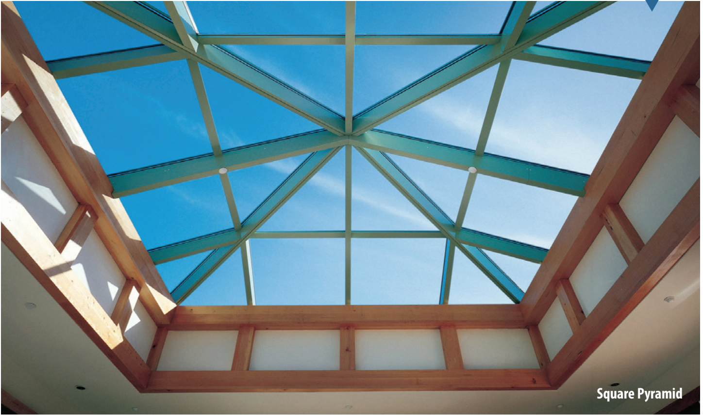
Not So Big Showhouse, Orlando, FL Pinnacle 600 Framing System, Pyramid, 16'6", 4:12 Pitch. Glazing: 1 1/8" IG. Finish: Kynar 500 Aged Copper.
