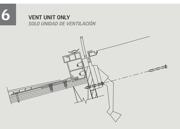
Attach the operator to the well framing with the two wood screws provided in the hardware kit.
