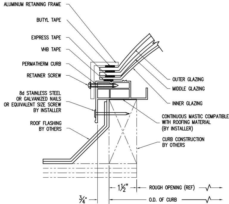
S.S. FASTENERS WILL BE REQUIRED IF PENETRATING PRESSURE TREATED WOOD
